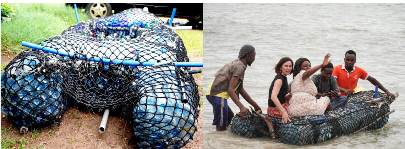
Picture 1: Left: A boat constructed by members of the Mtopanga River CBO using PET bottles collected from a public beach in Mombasa. Right: Conference participants testing the boat in coastal waters (Credit: CEJAD).
